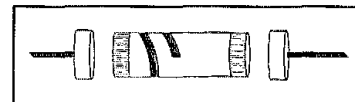
Fig 2—Details of film resistor construction, shown with end caps and leads removed. A spiral groove cut through the film and into the core trims the resistance to its final value. After spiraling, the resistor body and end caps are coated with resin, epoxy, or ceramic and labeled with the resistor's value.
